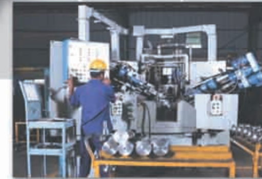
Oil Hole Drilling
