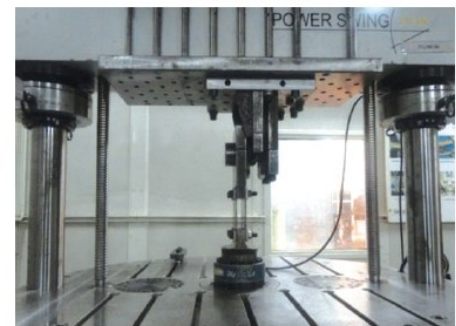
Fatigue Test (10 Million Cycles)
