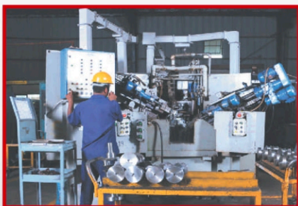
OIL HOLE DRILLING
